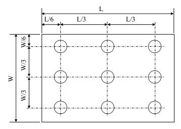
L max: The measured Maximum luminance of all measurement position.
