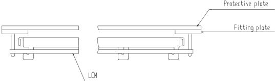
When assembling the LCM into other equipment, the spacer to the bit between the LCM and the fitting plate should have enough height to avoid causing stress to the module surface, refer to the individual specifications for
