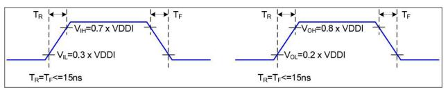
**Rising and Falling Timing for I/O Signal**
