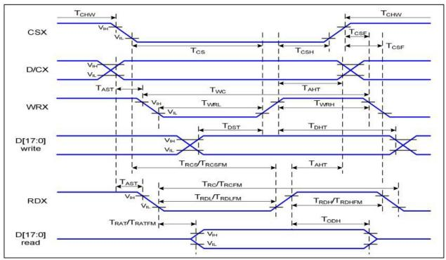
Parallel Interface Timing Characteristics (8080-Series MCU Interface)
