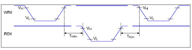
Write-to-Read and Read-to-Write Timing
