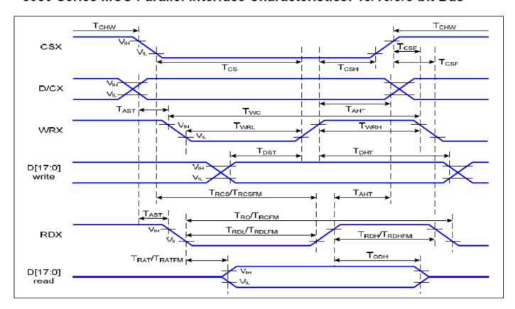
Parallel Interface Timing Characteristics (8080-Series MCU Interface)
