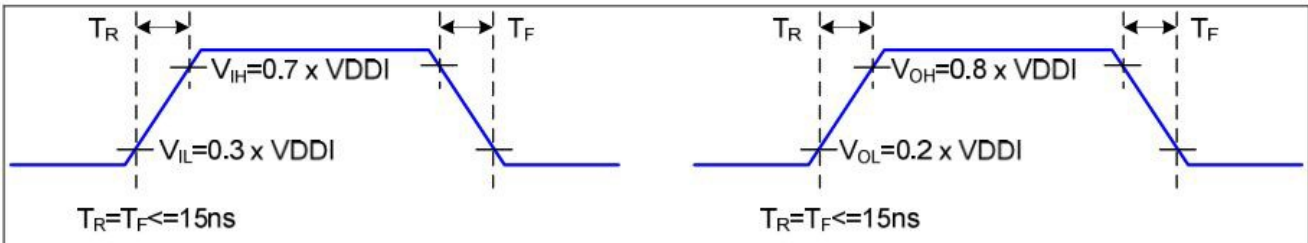
Rising and Falling Timing for I/O Signal
