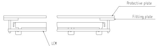
(2) When assembling the LCM into other equipment, the spacer to the bit between the LCM and the fitting plate should have enough height to avoid causing stress to the module surface, refer to the individual specifications for measurements. The measurement tolerance should be 0.1mm.
