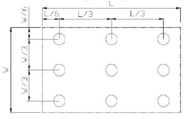
L max: The measured Maximum luminance of all measurement position. L min: The measured Minimum luminance of all measurement position.
