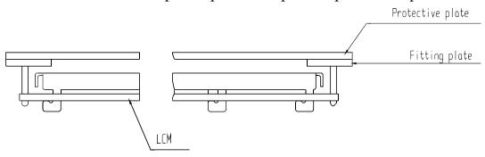
(2) When assembling the LCM into other equipment, the spacer to the bit between the LCM and the fitting plate should have enough height to avoid causing stress to the module surface, refer to the individual specifications for measurements. The measurement tolerance should be  $\pm 0.1$ mm.
