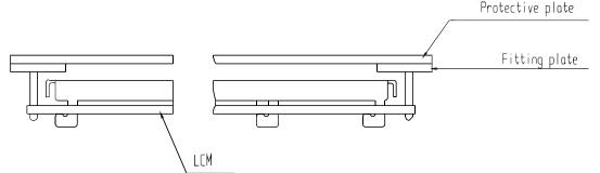
(2) When assembling the LCM into other equipment, the spacer to the bit between the LCM and the fitting plate should have enough height to avoid causing stress to the module surface, refer to the individual specifications for
