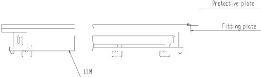
(2) When assembling the LCM into other equipment, the spacer to the bit between the LCM and the fitting plate should have enough height to avoid causing stress to the module surface, refer to the individual specifications for
