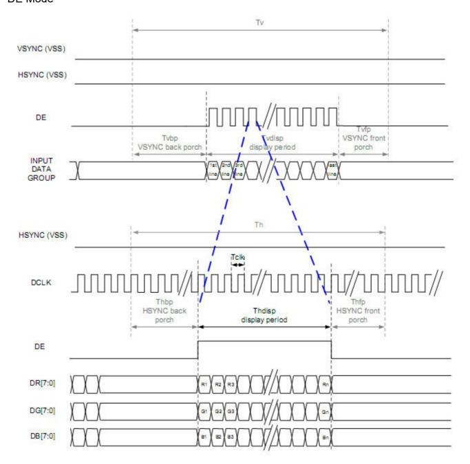
Parallel 24-bit RGB Input Timing
